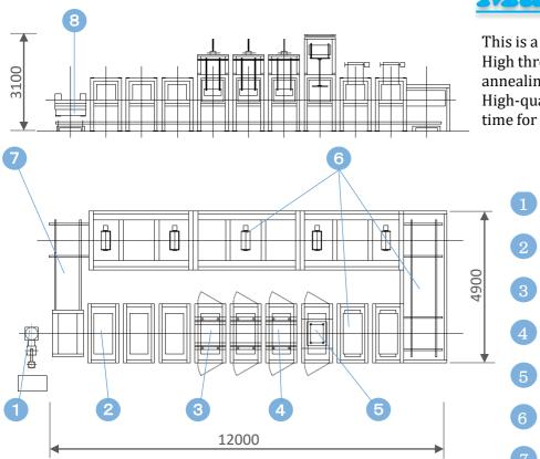
This is a small machine that performs preheating, bending, and annealing in a single furnace or a
