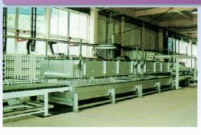
Air-cooled tempering equipment capable of producing tempered glass about three to five times that of ordinary flat glass. Can also be used for large sizes.
