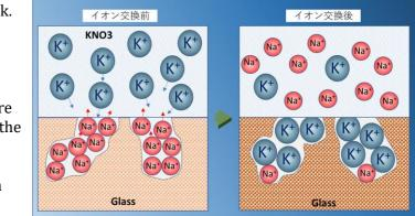
In the glass surface, Na+ is replaced by K+. According to the ion diameter, the compressive stress laver is formed.
